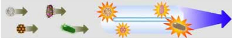
micro-organisms. Ultraviolet light possesses just the right amount of energy to break organic molecular bonds. As micro-organisms pass by the UV rays radiated from the ultraviolet lamp, this bond breakage translates into cellular or genetic damage for micro-organisms, such as germs, viruses, bacteria, fungi (like molds), etc. This results in the destruction of the
